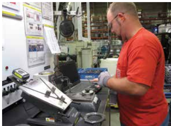
Shannon Gay performs a final inspection of the ID and Dog Tooth Depth on a Ford Super Duty Lock plate.
